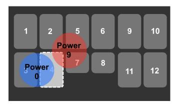
The pan with power level [9] is heated with induction coil 2, 4, 5 and 7.
